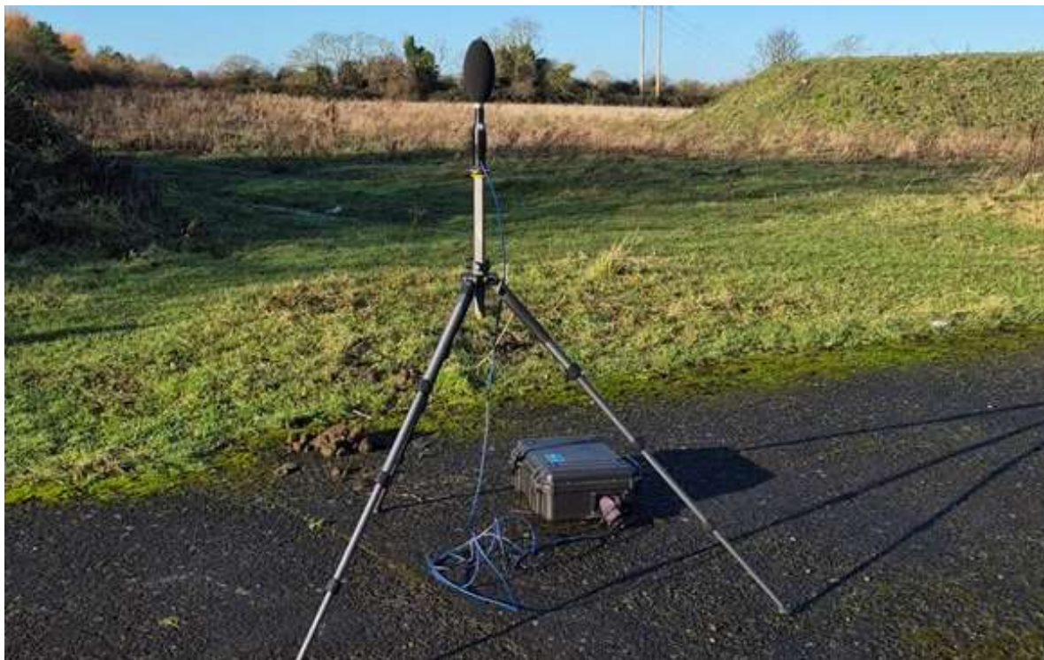
Figure 4.2: View of Noise Meter In-Situ During Baseline Survey
